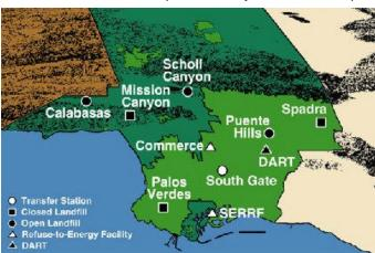
serving the needs of a large portion of Los Angeles County. This system includes three active sanitary landfills, two recycle centers, two transfer/materials recovery facilities, and three gas-to-energy facilities.
